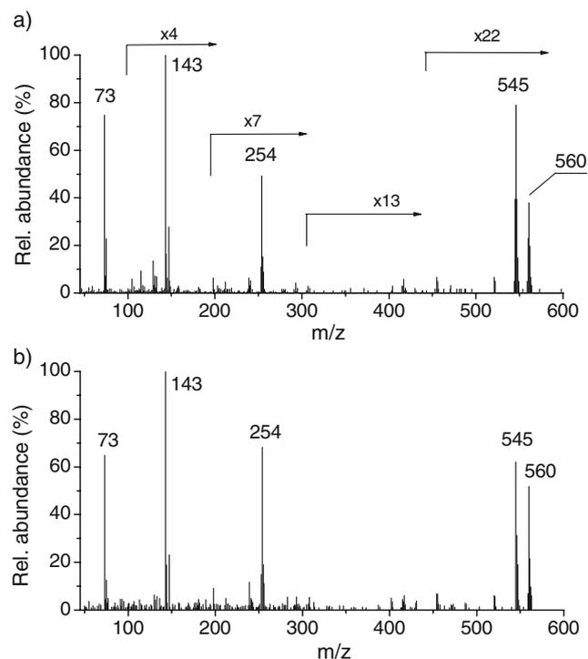
**Fig. 3** Comparison of **a** TOFMS spectra of 3'OH-stanozolol-3TMS acquired at  $0.5 \mu\text{g mL}^{-1}$  in standard solutions and **b** its entry from the NIST05 MS database. Note that the abundance of several consecutive mass intervals in TOFMS spectrum is enhanced by factors given above the intervals
