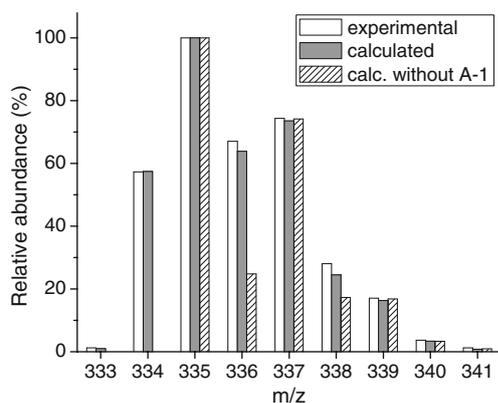
**Fig. 5** Cluster isotope pattern of clenbuterol-2TMS in standard solution at 0.5  $\mu\text{g mL}^{-1}$  for experimental data, calculated data by assuming the A-1 fragment has been formed in a ratio 1:2 against A and calculated data without taking the A-1 fragment formation into account
