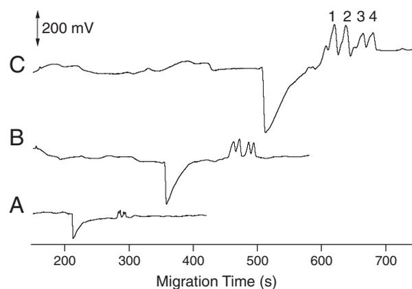
**Figure 1.** Electropherograms of a standard mixture of 50  $\mu$ mol/L of (+)-AP, (–)-AP, (+)-MA and (–)-MA separated in 150 mmol/L of acetic acid containing CMBCD at various concentrations: (A) 2 mmol/L, (B) 3 mmol/L, and (C) 4 mmol/L. Peaks: 1, (–)-AP; 2, (+)-AP; 3, (–)-MA; 4, (+)-MA.
