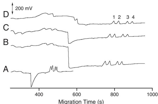
**Figure 2.** Electropherograms of a standard mixture of 50  $\mu\text{mol/L}$  of (+)-AP, (-)-AP, (+)-MA and (-)-MA separated in 150 mmol/L of acetic acid containing 3 mmol/L of CMBCD and HPMC at various concentrations: (A) 0 (% w/v), (B) 0.1 (% w/v), (C) 0.2 (% w/v), and (D) 0.3 (% w/v). Peaks: 1, (-)-AP; 2, (+)-AP; 3, (-)-MA; 4, (+)-MA.
