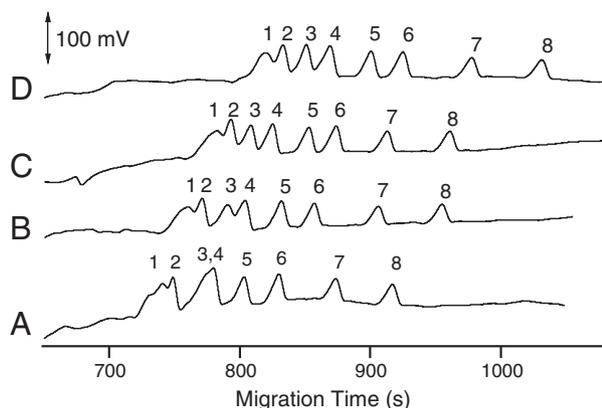
**Figure 3.** Electropherograms of a standard mixture of 50  $\mu\text{mol/L}$  of (+)-EP, (-)-EP, (+)-PE, (-)-PE, (+)-NE, (-)-NE, (+)-NPE, and (-)-NPE separated in 150 mmol/L of acetic acid containing 0.2 (%w/v) of HPMC, 3 mmol/L of CMBCD and DMBCD at various concentrations: (A) 0 mmol/L, (B) 2 mmol/L, (C) 3 mmol/L, and (D) 4 mmol/L. Peaks: 1, (-)-NPE; 2, (+)-NE; 3, (-)-NE; 4, (+)-PE; 5, (+)-EP; 6, (-)-EP; 7, (+)-NPE; 8, (+)-PE.
