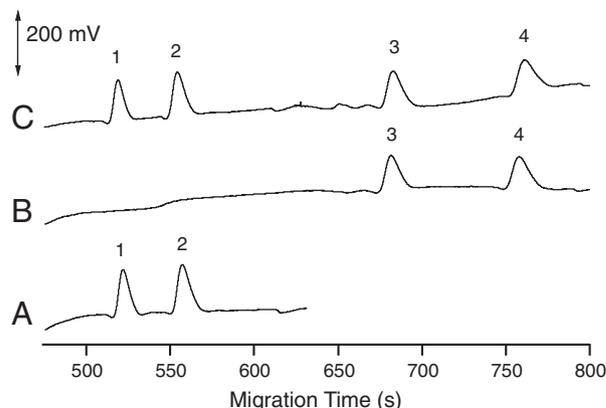
**Figure 4.** Electropherograms (inverted signal) of (A) a standard mixture of 100  $\mu\text{mol/L}$  of (+)-NPE, and (-)-NPE, (B) a standard mixture of 100  $\mu\text{mol/L}$  of (+)-NE, and (-)-NE, and (C) a standard mixture of 100  $\mu\text{mol/L}$  of (+)-NE, (-)-NE, (+)-NPE, and (-)-NPE separated in 500 mmol/L of acetic acid containing 5 mmol/L of DMBCD and 5 mmol/L of 18C6H<sub>4</sub>. Peaks: 1, (+)-NPE; 2, (-)-NPE; 3, (-)-NE; 4, (+)-NE.
