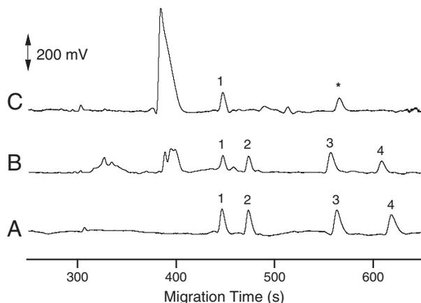
**Figure 6.** Electropherograms (inverted signal) of (A) a standard mixture of (+)-NE, (-)-NE, (+)-NPE, (-)-NPE, (B) the extracted blank urine sample spiked with a standard mixture of (+)/(-)-NE, (+)/(-)-NPE, (+)/(-)-EP, (+)/(-)-PE, (C) the extracted urine sample **C** separated in 500 mM acetic acid containing 5 mmol/L of DMBCD and 5 mmol/L of 18C6H<sub>4</sub>. Peaks: 1, (+)-NPE; 2, (-)-NPE; 3, (-)-NE; 4, (+)-NE.
