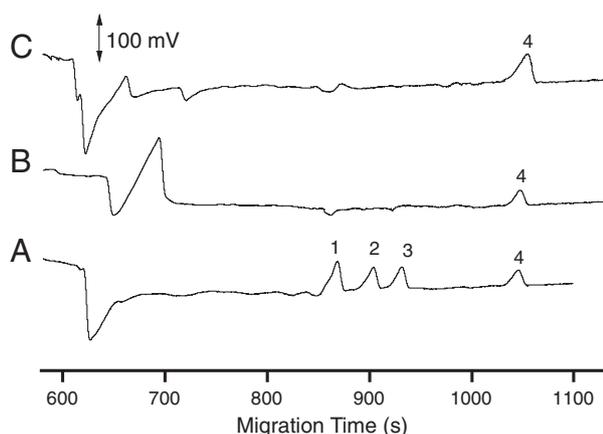
**Figure 7.** Electropherograms of (A) a standard mixture of (+)-EP, (-)-EP, (+)-PE, (-)-PE, (B) the extracted urine sample **D**, (C) the extracted urine sample **C** (diluted 10 times) separated in 150 mmol/L of acetic acid containing 0.2 (% w/v) of HPMC, 3 mmol/L of CMBCD, and 3 mmol/L of DMBCD. Peaks: 1, (-)-PE; 2, (+)-EP; 3, (-)-EP; 4, (+)-PE.
