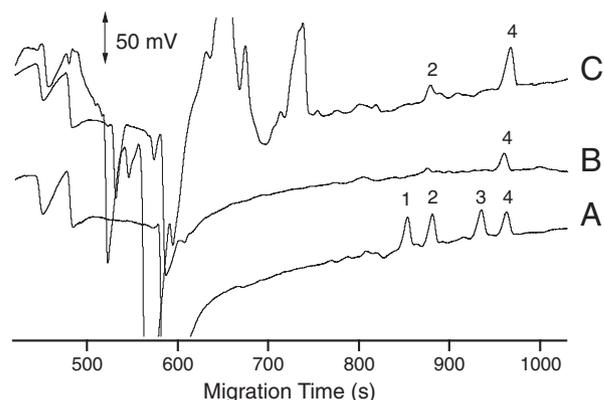
**Figure 5.** Electropherograms of (A) a standard mixture of (+)-AP, (-)-AP, (+)-MA, (-)-MA, (B) the extracted urine sample A, (C) the extracted urine sample B separated in 150 mmol/L of acetic acid containing 0.2 (% w/v) of HPMC and 3 mmol/L of CMBCD. Peaks: 1, (-)-AP; 2, (+)-AP; 3, (-)-MA; 4, (+)-MA.
