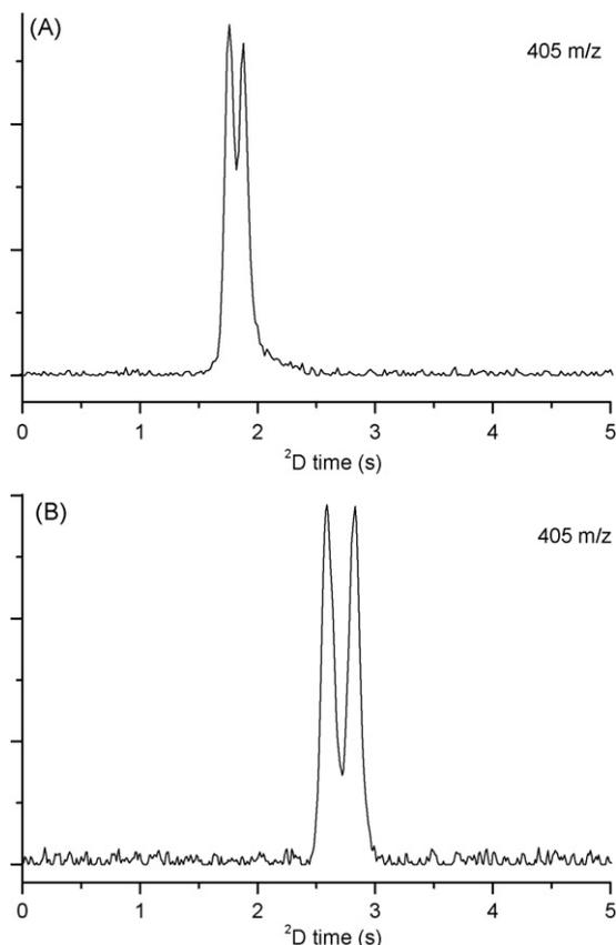
**Fig. 5.** Extracted ion chromatogram at  $405 m/z$  for 19-norandrosterone, showing the achieved separation from the co-eluting endogenous component on  $0.1 \mu\text{m}$  (A) and  $0.2 \mu\text{m}$  (B)  $d_I$  2D column. (2) is the first eluting peak.
