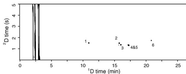
**Fig. 2.** GC  $\times$  GC-FID contour plot of the TMS derivatized WADA “key” AA on BPX5/BPX50 column configuration: (1) clenbuterol, (2) 19-norandrosterone, (3) epimethendiol, (4) M1 metabolite, (5) M2 metabolite, and (6) 3’OH-stanozolol.
