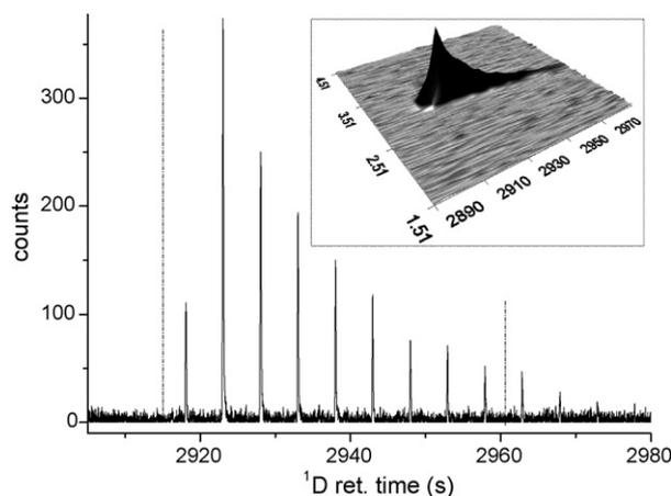
Fig. 9. Extracted ion chromatogram at 254 *m/z* of 3-OH-stanozolol at 10 ng mL<sup>-1</sup> in standard solution showing the <sup>1</sup>*t<sub>R</sub>* range in which 9 modulations were detected and integrated automatically by ChromaTOF software. The extracted 3D plot in the inset shows the integrated surface.
