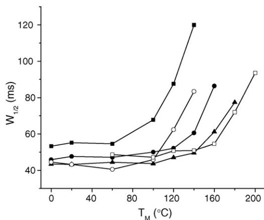
**Fig. 3.** The influence of modulator temperature ( $T_M$ ) on peak width ( $w_{1/2}$ ) for the WADA “key” AA. Clenbuterol (■); 19-norandrosterone (●); epimethendiol (▲); M2 metabolite (○) and 3’OH-stanozolol (□).
