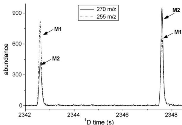
Fig. 8. Mass spectral deconvoluted modulated peaks for ions 255 and 270 *m/z*, corresponding to M1 and M2 metabolites, in a standard solution, showing that the peaks strongly overlap on both the first and second columns.
