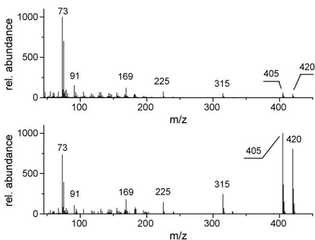
**Fig. 10.** The comparison of TOFMS spectrum of 19-norandrosterone recorded at  $1 \mu\text{g mL}^{-1}$  in standard solution (A) to its entry in NIST05 quadrupole MS-based library (B).
