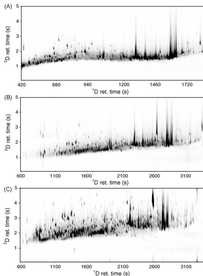
**Fig. 4.** 2D plots of spiked urine extracts with the WADA key AA at a concentration of  $2 \text{ ng mL}^{-1}$ , analyzed under NP/P1<sub>S</sub> (A), NP/P1<sub>L</sub> (B) and NP/P2<sub>L</sub> (C) chromatographic conditions.
